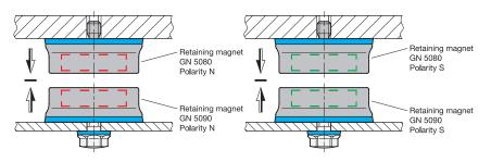
Combining two retaining magnets with the same polarity creates a repelling force.
